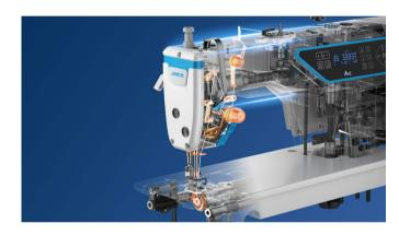
• **O - degree Thread Path Technology:** Precise thread handling • Precise thread catching Jack's exclusive thread - passing technology reduces thread tension by **30%**.
