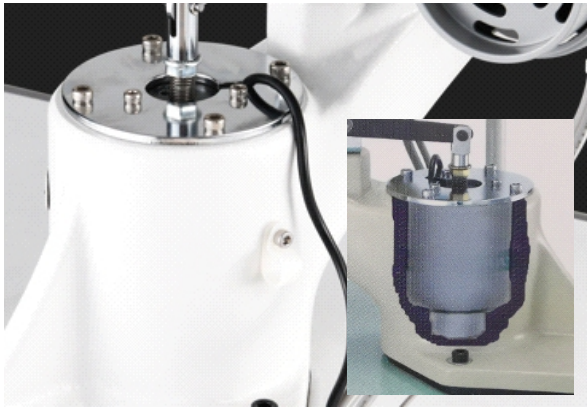
Standard automatic presser foot lifter, high efficiency
