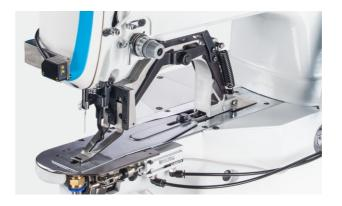
6 Thread Remaining Tacking and Cleanness No need manual trimming. High efficiency
