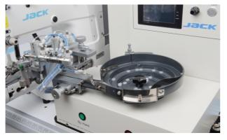
5 Automatic Button Feeding Device, High Efficiency(JK-T1903GR)
