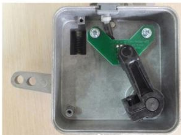
Picture 9 the position when motor stop running
